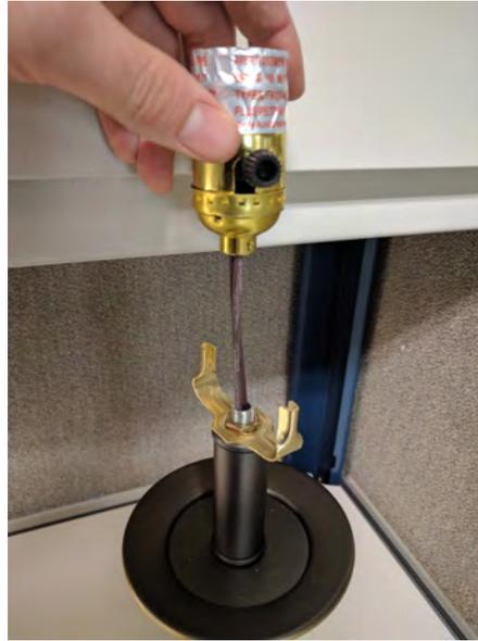
IV. The socket's electrical cord should now be visible, use wire cutters to cut the cord and separate the socket from the lamp.
