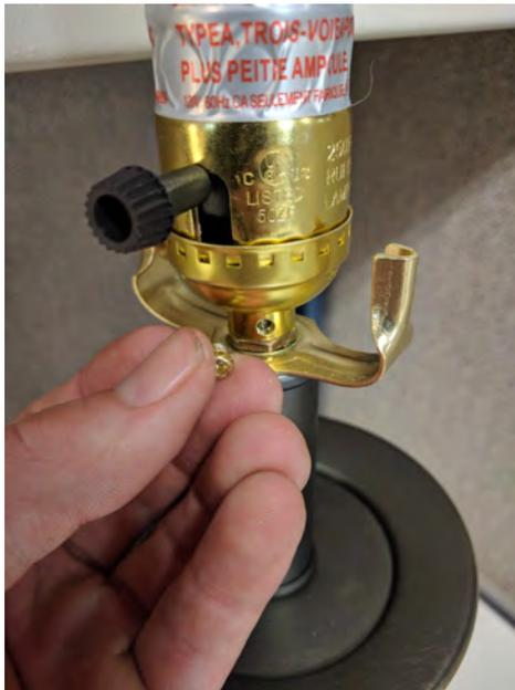
III. Twist the socket counterclockwise to remove it.
