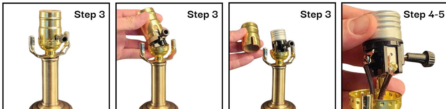
5- Loosen set screw and twist counterclockwise to remove socket base from lamp. *If your lamp does not have a set screw, it could have adhesive on the threads which may require a heat gun to loosen.*
